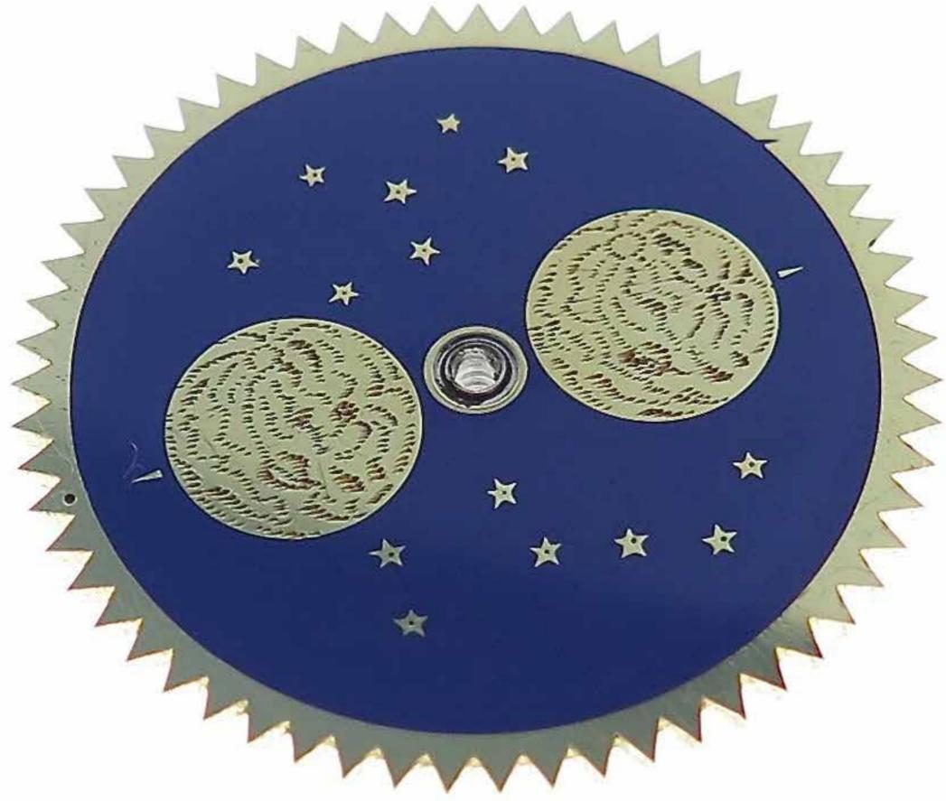
The gold moon phases wheel with blue enamel, and hand engraved texture. The punched "dot" at 9 oʻclock was for aligning the wheel to a specific datum point when it was first assembled on the module prior to the dial being added.
